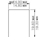
Single Panel - Latch Clearance Panel Thickness 0.062 inch
